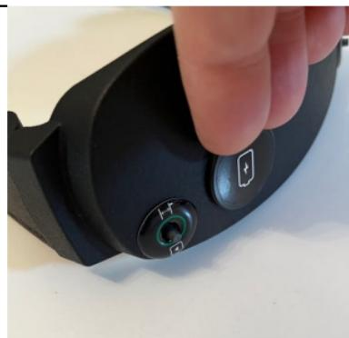
To loosen the plug that closes the access to the battery, position the fingernails of two fingers in the gap between the plug and the glasses as in the picture.
