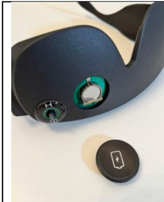
Once you remove the plug, you will see the button cell type CR 1220 3V (3.0 volt button cell DL1220 / CR1220 / CR 1216. Note: CR 1225 will not fit because it is too thick).
