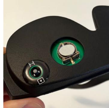
To insert the new button cell type CR 1220 3V, hold the glasses horizontally as shown in the picture and position the button cell loosely on the button cell holder; plus contact facing up.
