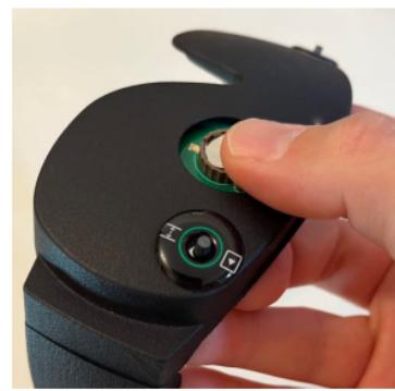
Press the button cell carefully and with extremely little force into the button cell holder until it clicks into place and cannot fall out. Please note that too much pressure could damage the glasses.
